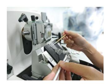
Paraffin is one of the most used products in laboratories of Anatomic Pathology. The paraffin blocks are placed on a device that uses an extremely sharp knife (a microtome) to obtain very thin pieces of tissue.
